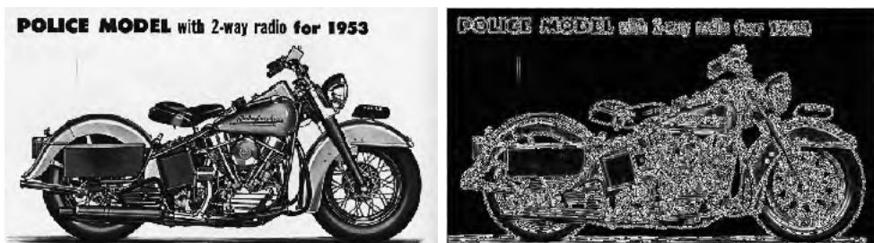
Figure 3.5.1. Motorcycle and the image that represents the magnitude component of the Prewitt edge detector.
