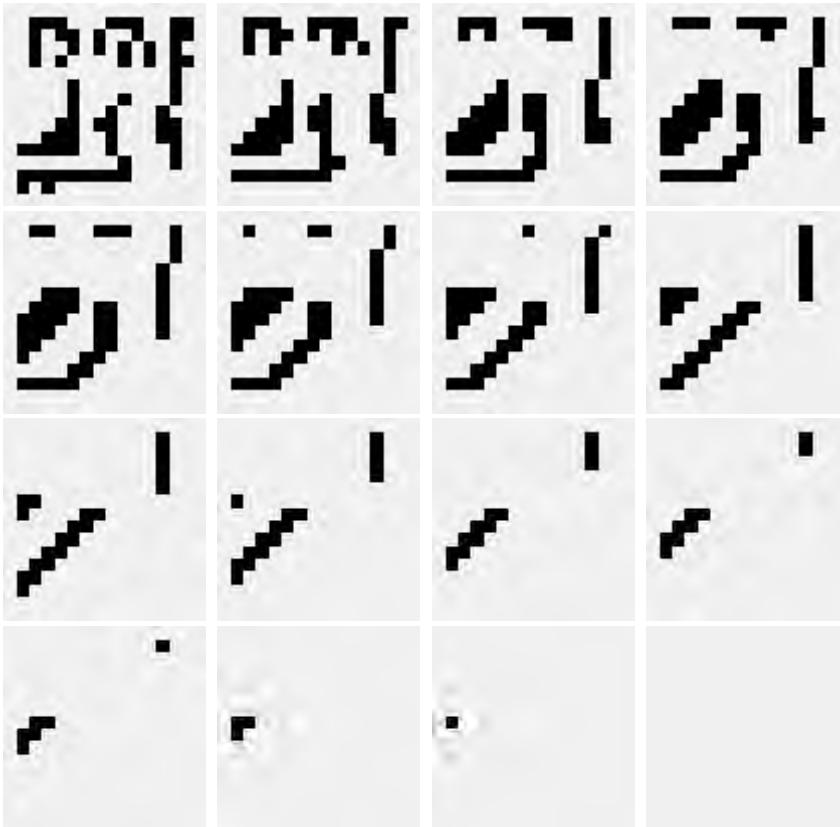
Figure 6.4.1. The parallel shrinking process.
