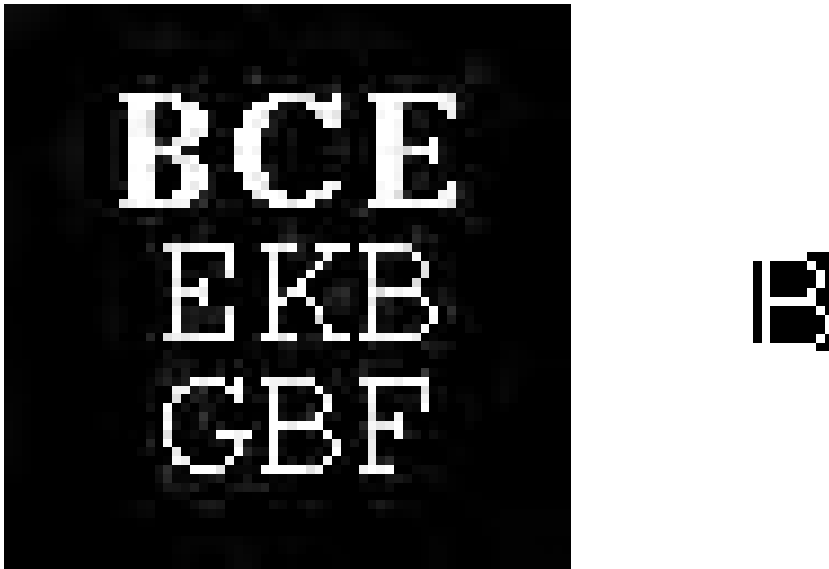
Figure 9.3.1. The input image \mathbf{a} is shown on the left and the pattern template \mathbf{t} on the right.
